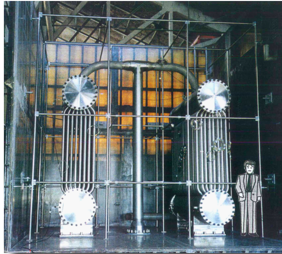
Figure 4-7 PCCS Heat Exchanger Testing
