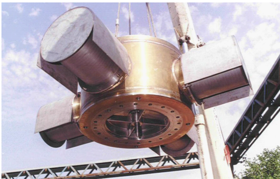
Figure 8-18. Prototype Vacuum Breaker
