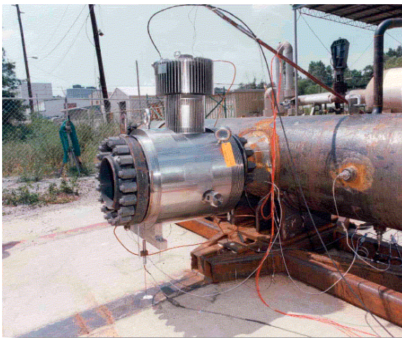
Figure 3-11. DPV Under Test
