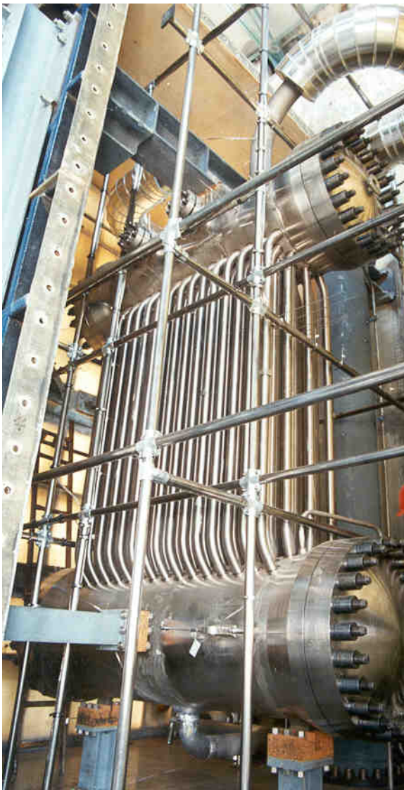
Figure 3-14. Isolation Condenser Test Module
